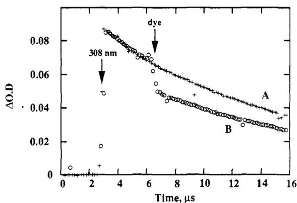
Figure 3. Decay of transients produced from  $\alpha$ -chloro-2',5'-dimethylacetophenone in methanol, monitored at 380 nm for 308-nm excitation (trace A) and 308-nm excitation followed by a 420-nm laser pulse (trace B).
