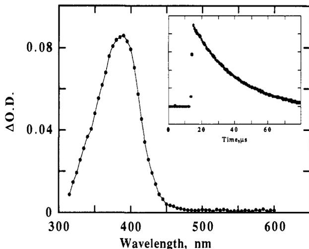
Figure 1. Transient absorption spectrum obtained on 308-nm excitation of 1 mM  $\alpha$ -chloro-2',5'-dimethylacetophenone in methanol. Insert: Decay trace at 380 nm due to the *E* enol generated as above.
